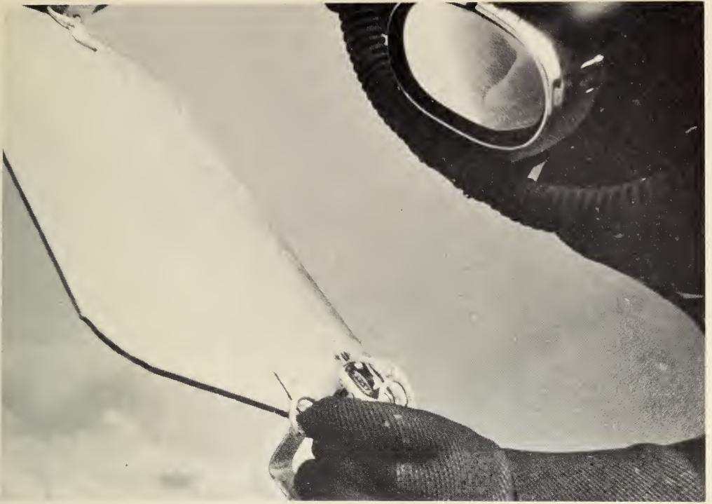
A research diver uses a "counting board", a simple recording device to estimate the abundance of several species of plankton at the same time.
